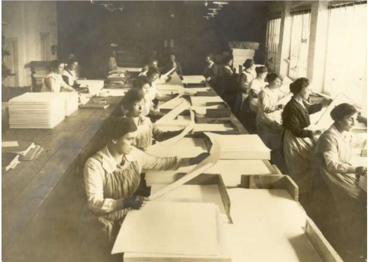
The sheets are examined, counted twice, and then packed up in reams, each ream being sealed with a special government seal.
