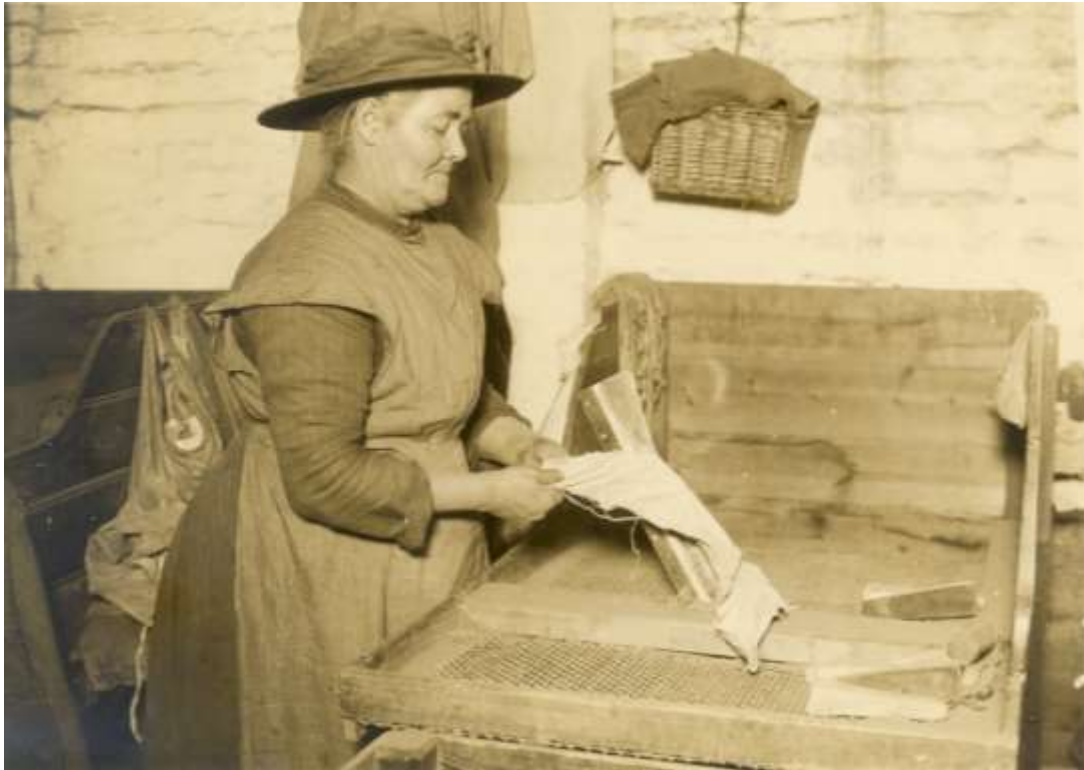
Cutting up and sorting the rags; the best cotton ones are selected for the stamp paper, as paper made from them is kindest to the printing plates.
