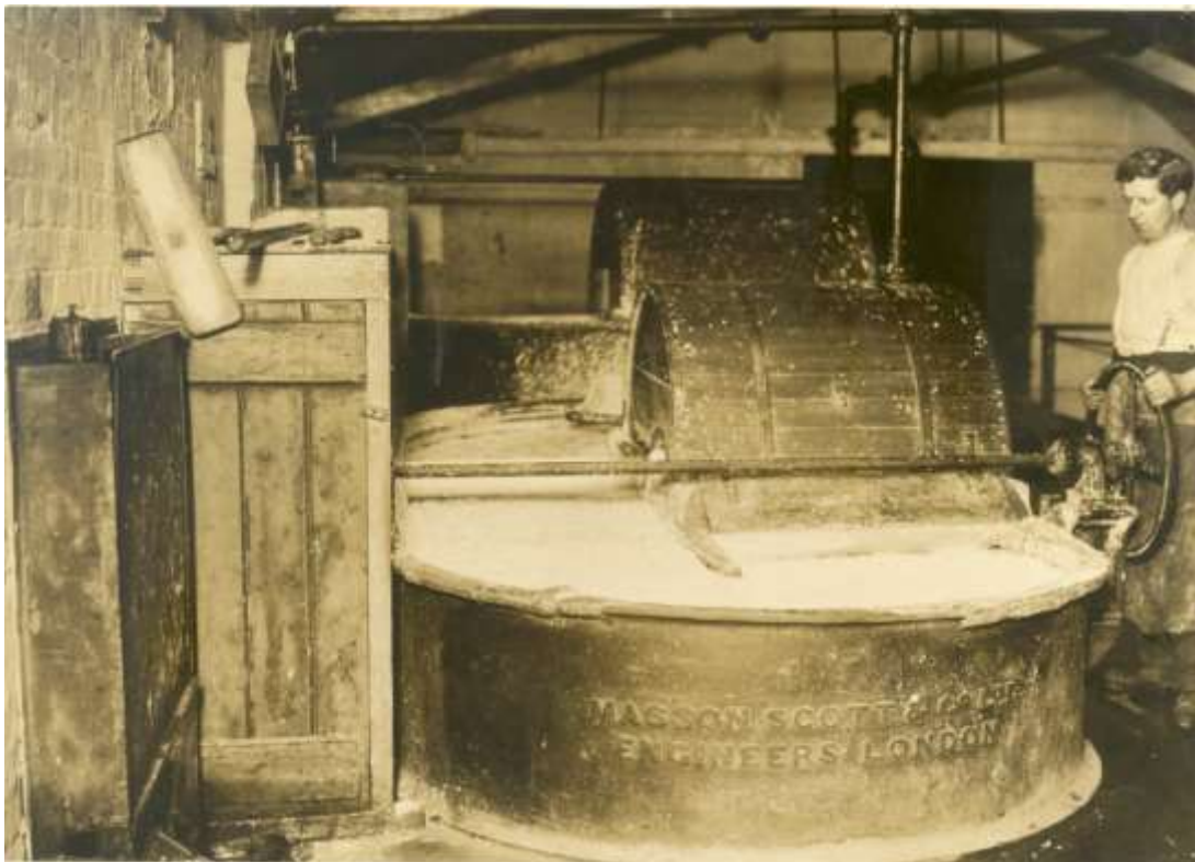
In the beater the "half-stuff" is ground under a heavy roller to disintegrate and hydrate every fibre.
